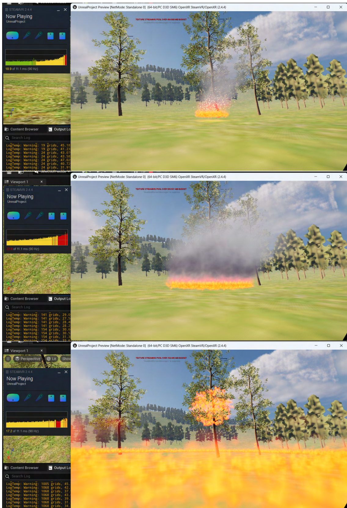
Figure 5.6: The fire particles, at full quality, smoke and flames only, and tall flames only respectively. Screenshots were taken once the performance had degraded past 16.6 ms.
